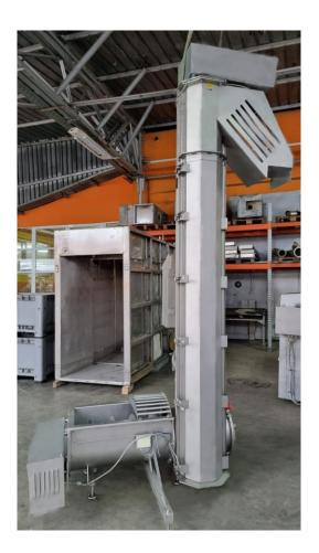
Designed for vertical conveying of fresh or cooled minced meat and wide range of loose materials. Conveying is done through a feeding horizontal screw and a vertical screw. Activation is done by directly connected reduction gear motors. The vertical screw has covers for easy cleaning. With a possibility to be included in production lines.
